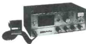
New Model 712 — Sentinel 12 Dual Conversion 5-watt CB Transceiver. Permits 12-channel crystal-controlled transmit and receive, plus 23-channel tunable receive. Incorporates adjustable squelch & noise limiter, & switches for 3.5 watt P.A. use, spotting, & Part 15 operation. Transistorized 12VDC & 117VAC dual power supply. $99.95 wired only.
